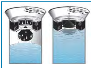
Floor drain float plug.
